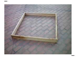
After the boards are nailed together (like it is shown above) paint the outside using white latex paint. This provides protection for the wood from water, light, bacterial and fungal damage. Now line the frame with the plastic, nailing it on the borders using small nails.
