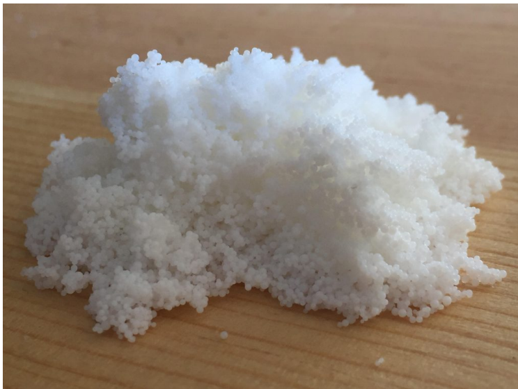
A weakly acidic ion-exchange resin used for pH control
