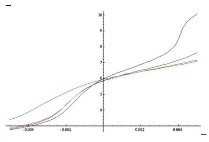
The blue curve represents the behavior of a poorly buffered hydroponic solution with only about 0.002M phosphate concentration (about 50 ppm of P). The red and yellow curves represent two solutions with increasing levels of carbonate showing us that if you are battling pH increases, having more
