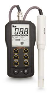
As in the case of pH meters the correct calibration of an EC meter ideally requires the use of two solutions. Most people however use only one solution or use two solutions in a
