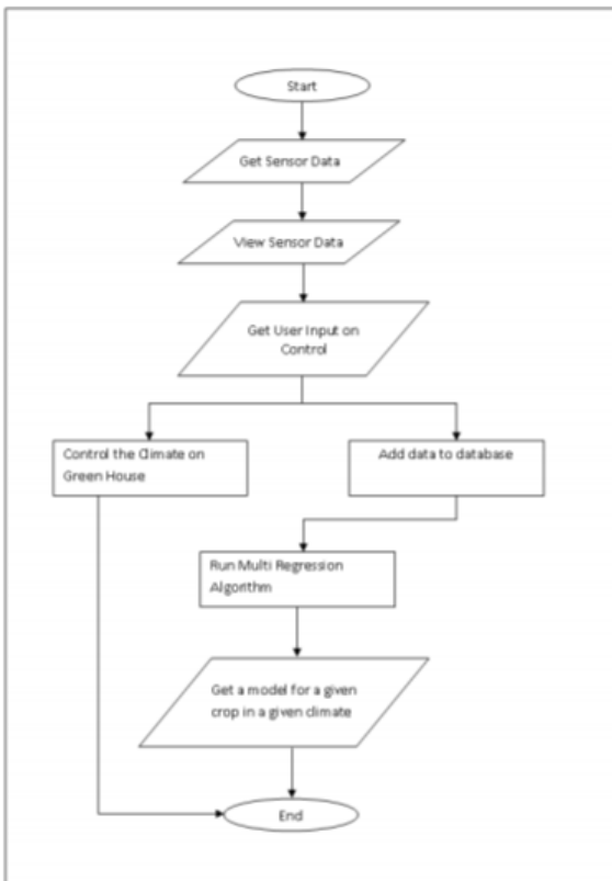
Fig. 11. Overall process of the System
