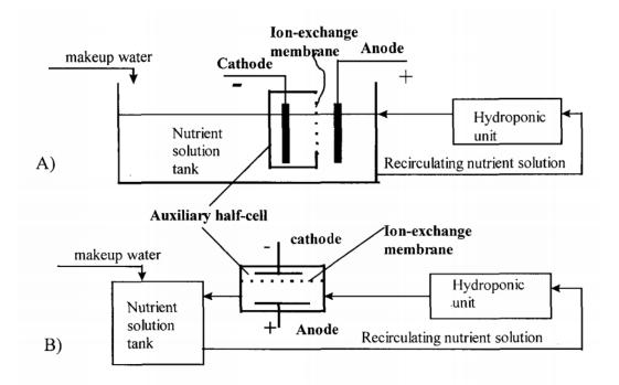
Image taken from <u>this paper</u>, which discussed the topic of electrochemical pH control in hydroponic systems at length. One of the big challenges of this setup is that the cathode
