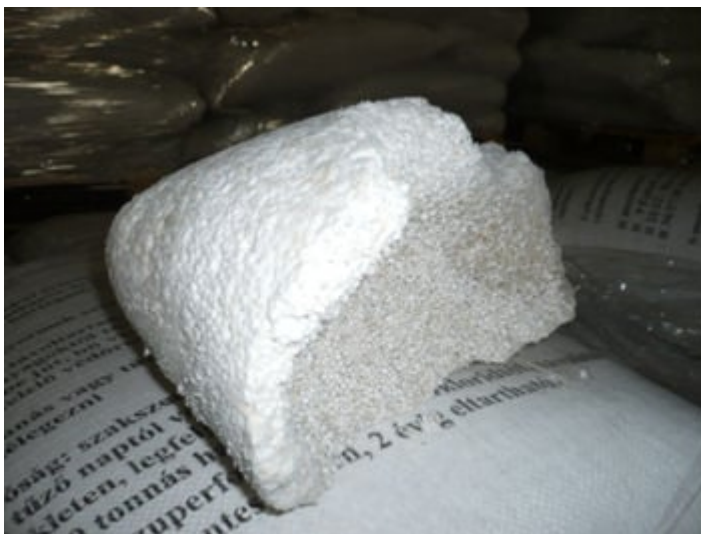
Caking of a fertilizer product due to a reaction with atmospheric water
