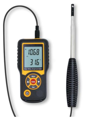
A hot wire anemometer that can be used to accurately measure wind speeds around plant canopy
