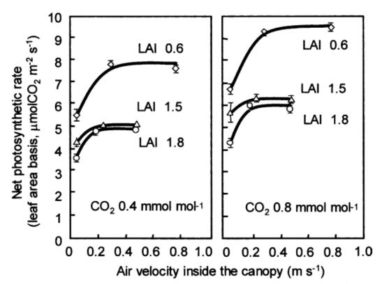
Photosynthetic rate as a function of windspeed, LAI stands for (Leaf Area Index). Taken from <u>this article</u>.
