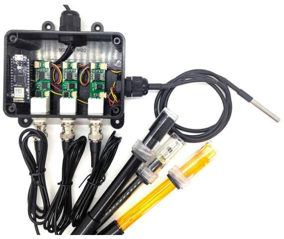
A custom built data logging system to read EC/pH/ORP. Read more here.
