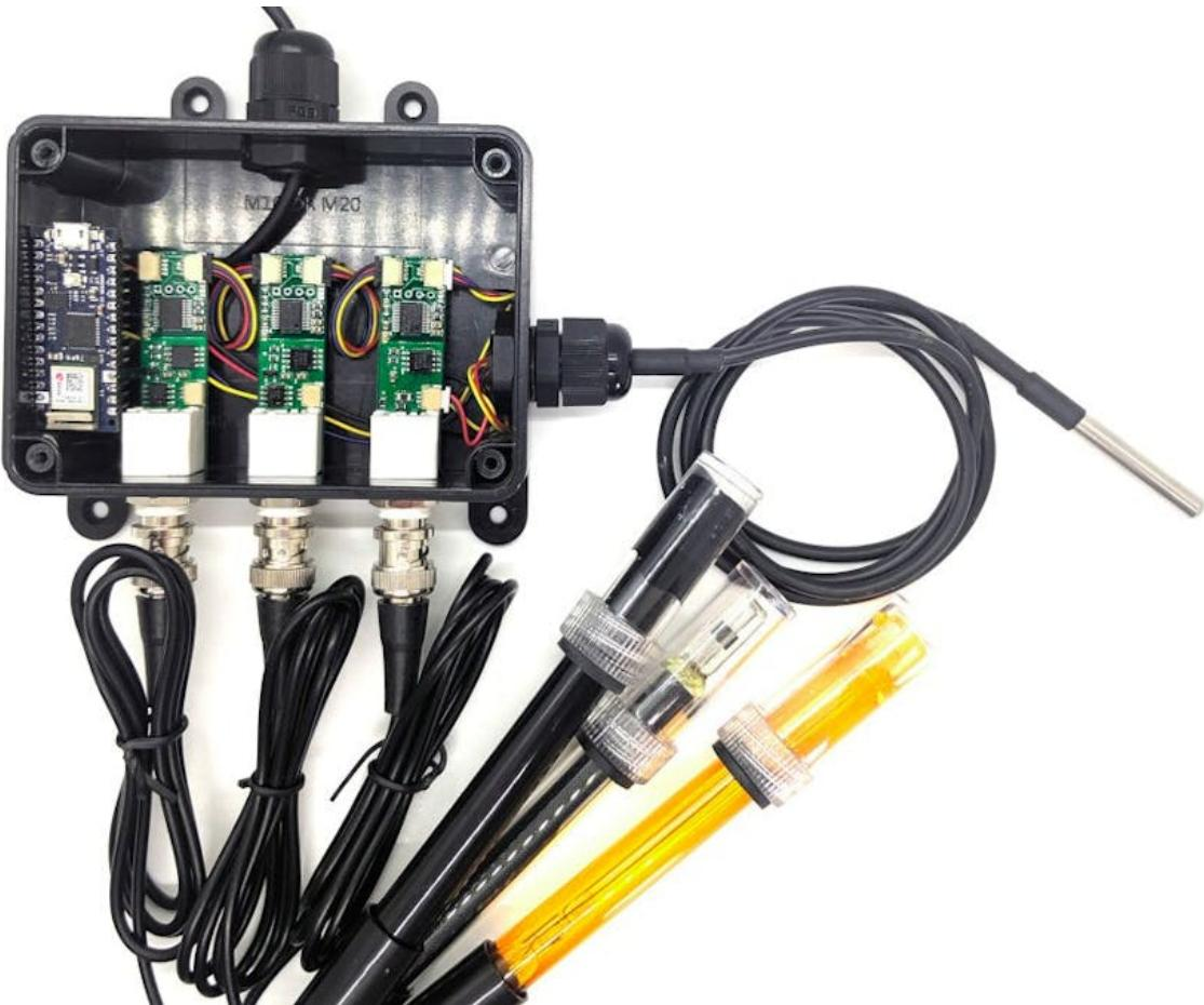
A custom built data logging system to read EC/pH/ORP. Read [more here](#).
