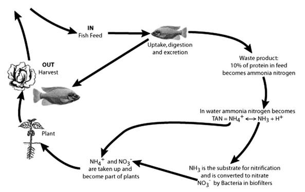
Basic process diagram of an aquaponic setup (from <a href="here">here</a>)
