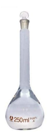
Volumetric flasks can be used for highly accurate small scale preparations
