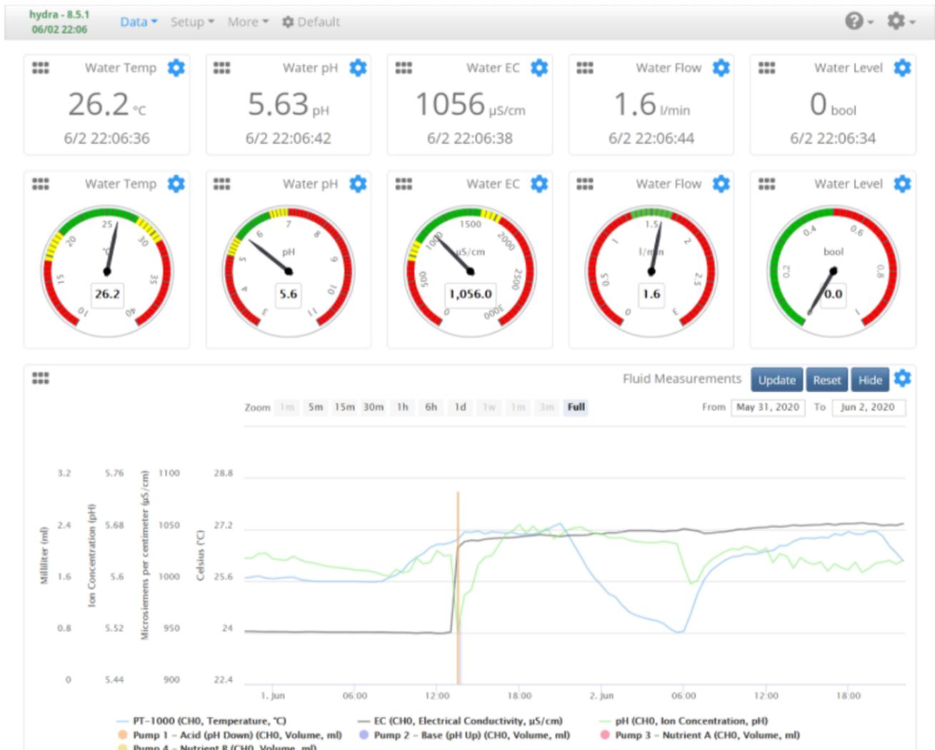
A sample of the data-logging capabilities of a MyCodo server. Taken from the [MyCodo site](#).
