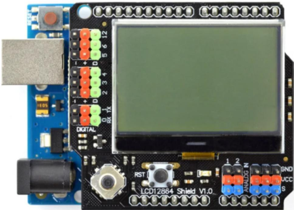
The LCD12864 Gravity shield that exposes easy plug-and-play ports for sensors
