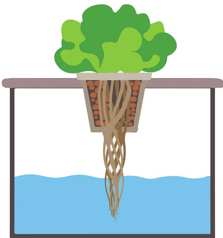
A traditional Kratky setup. Note that the solution at the bottom is stagnant and not actively oxygenated in anyway. Only the oxygen that diffuses from the air gets into the water. This is enough to keep the submerged roots alive, provided that the solution itself does not act as a sink for oxygen. In these cases, root rot is quickly experienced.
