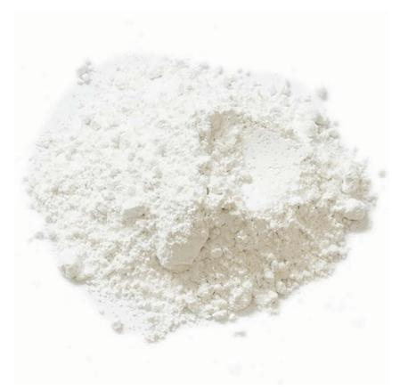
Vansil CS-1, one of the most common forms of calcium silicate (wollastonite) used as an amendment in soilless crops.
