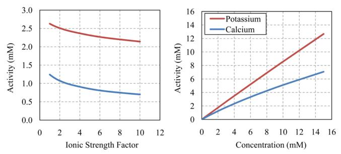
Activity versus concentration for monovalent potassium  $(K^+)$  and divalent calcium  $(Ca^{2+})$  in half-strength Hoagland nutrient solution. The left panel shows how ionic activity declines as solution ionic strength increases, with divalent calcium affected far more severely than monovalent potassium. The right panel demonstrates that activity diverges substantially
