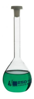
Picture of a type A 250mL volumetric flask.
