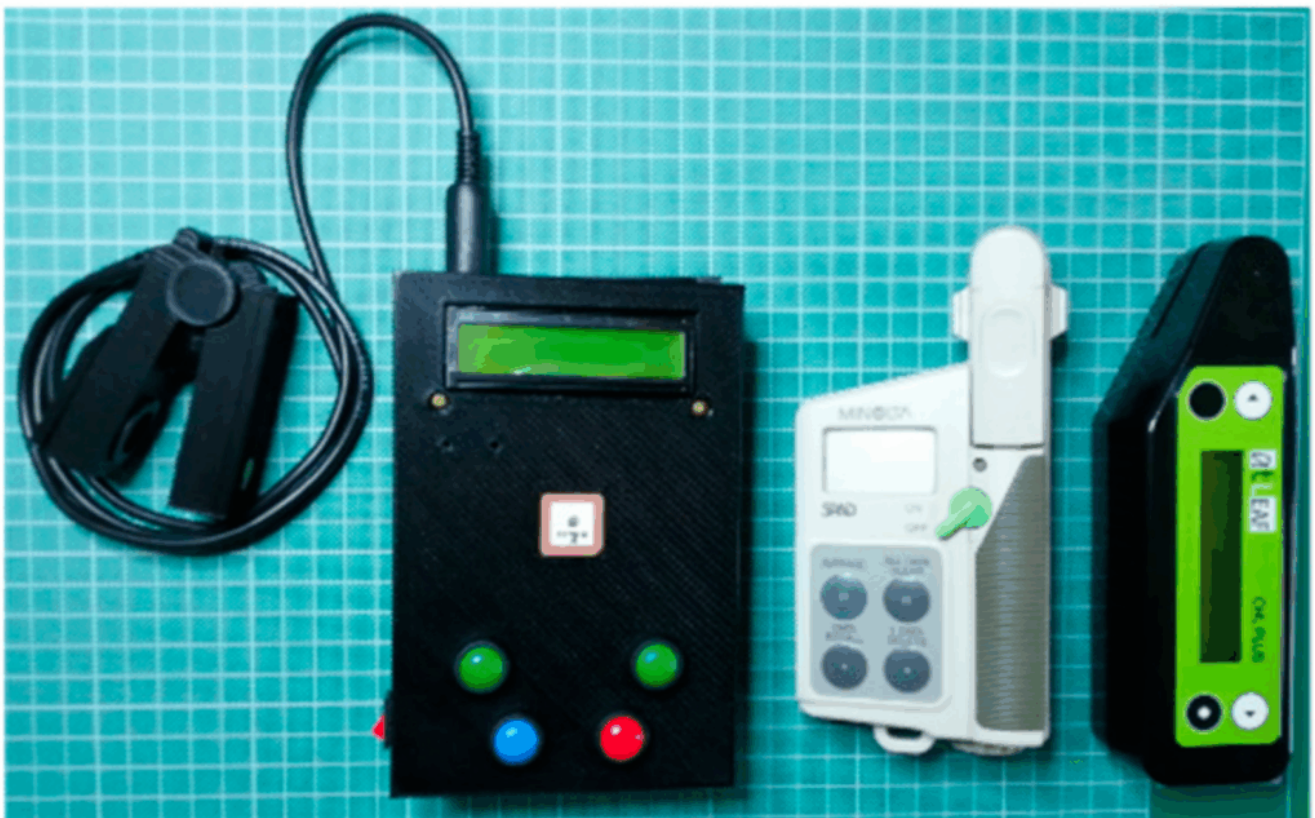
A DIY chlorophyll meter compared to some commercial alternatives (taken from ( 9 )).
