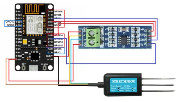
Diagram showing cable connections between moisture content sensor NodeMCUv3 and communication board.
