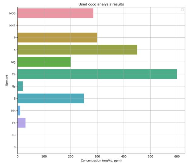
Analysis of used coco from a tomato crop. This analysis uses a DTAP + ammonium acetate process to extract all nutrients from the media. This media had a runoff pH of 6 with an EC of 3.0 mS/cm.
