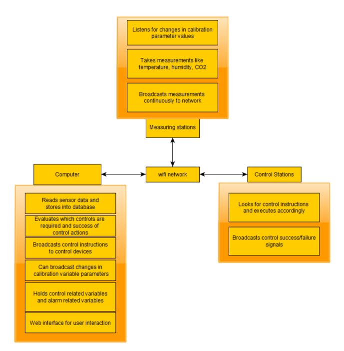
Usual network configuration I used to built electronic monitoring/control infrastructures for hydroponics
