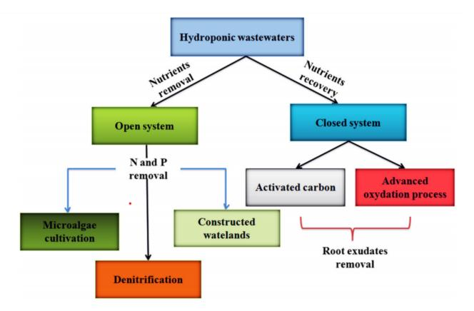
Route for the treatment of hydroponic waste waters depending on whether nutrients are to be removed or recovered (taken from the review mentioned above). Note that eventually solutions need to be changed so the disposal of nutrient solutions cannot be endlessly avoided, even in close systems.
