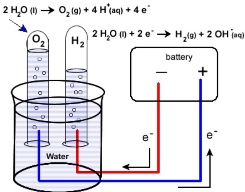
The image above shows the half reactions involved in the oxidation (left) and reduction (right) of water.
