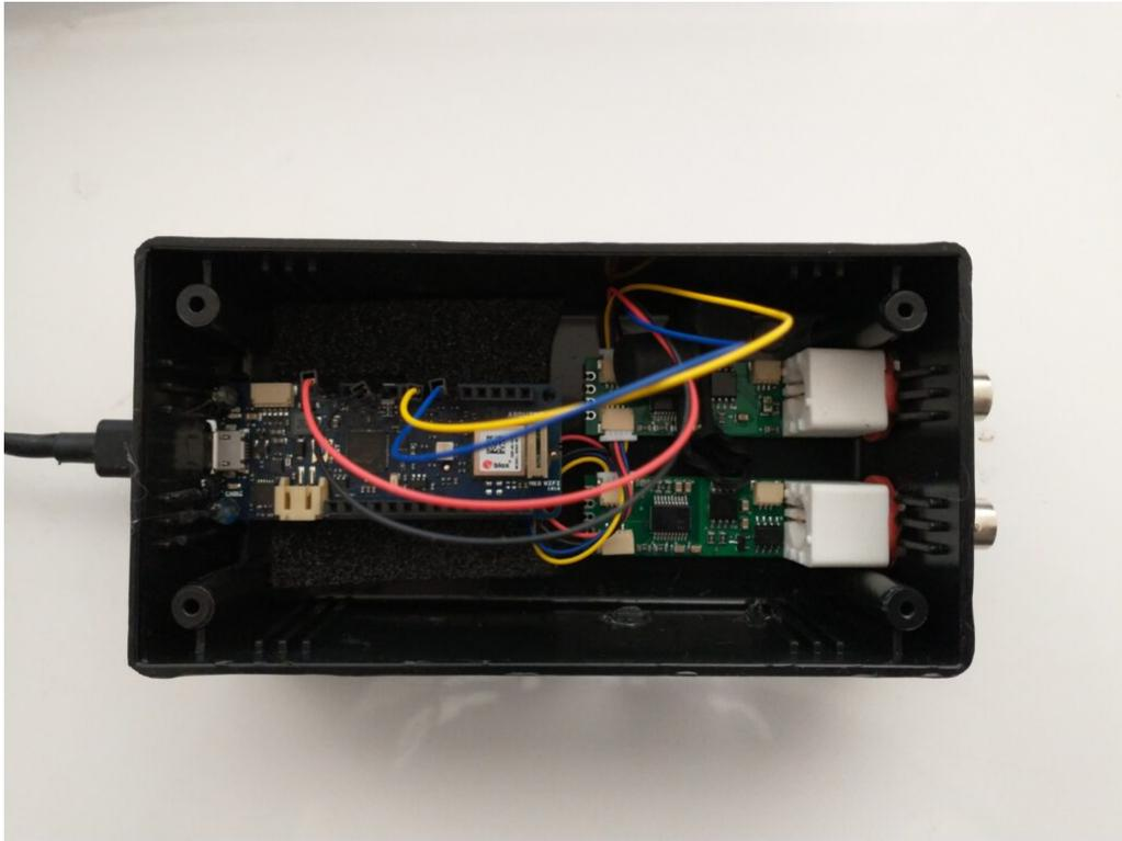
My Arduino MKR wifi 1010 based sensing station, using uFire pH and EC boards in a small project box.
