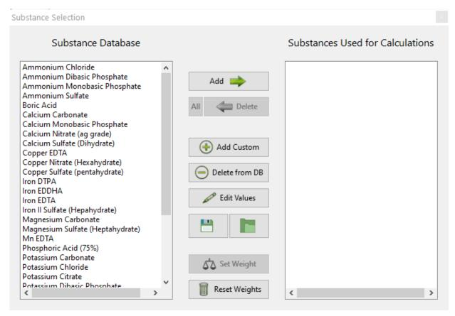
The HydroBuddy "Substance Selection" screen (v1.8) showing some of the nutrients in the default database
