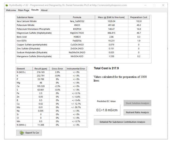
Standard Hoagland solution calculation using HydroBuddy with a set of basic chemicals.
