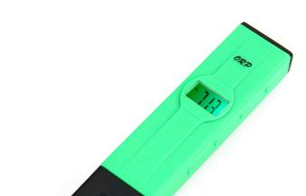
An ORP meter or "Oxidation-Reduction Potential" meter characterizes the electrochemical environment within a solution. An ORP meter has two electrodes, a traditional reference electrode with a known potential and a platinum electrode whose potential changes depending on how hard the solution is pushing either to take electrons from the platinum electron or give it electrons. A solution that has a lot of substances that are willing to give electrons will tend to
