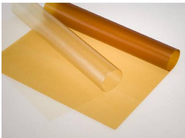
A modern anion exchange membrane. Fundamental to the idea of an electricity-only pH control system
