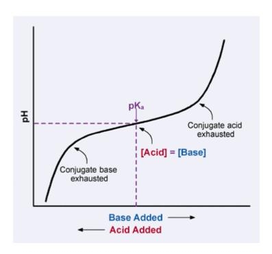
What we are doing with the above procedure is basically adding two acidic substances which have pKa values close the pH values that interest us. Close to 7 (mono basic phosphate) and close to 4 (citric acid). We then generate the necessary amount of conjugate base to reach the necessary pH level by adding KOH. The buffer strength is established by the initial amount of the acidic substance we add and the role of the KOH
