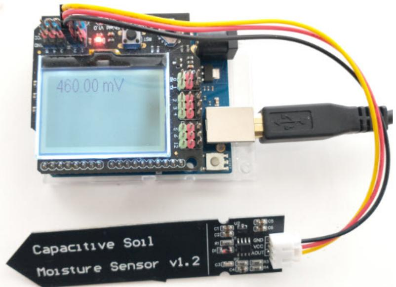
An Arduino Wifi Rev2 connected to a moisture sensor, transmitting readings to an MQTT server hosted by flespi that generates an online dashboard
