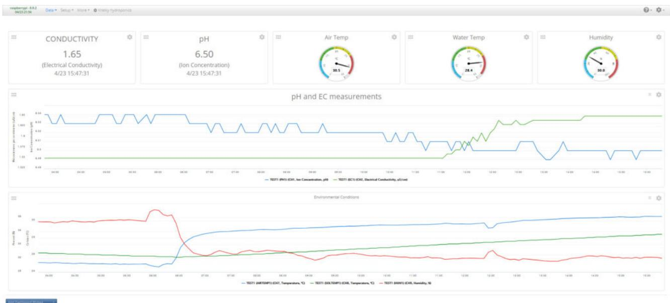
The dashboard of my MyCodo server, showing the measurements of the system as a function of time. All readings are also recorded in the MyCodo database for future reference and processing.
