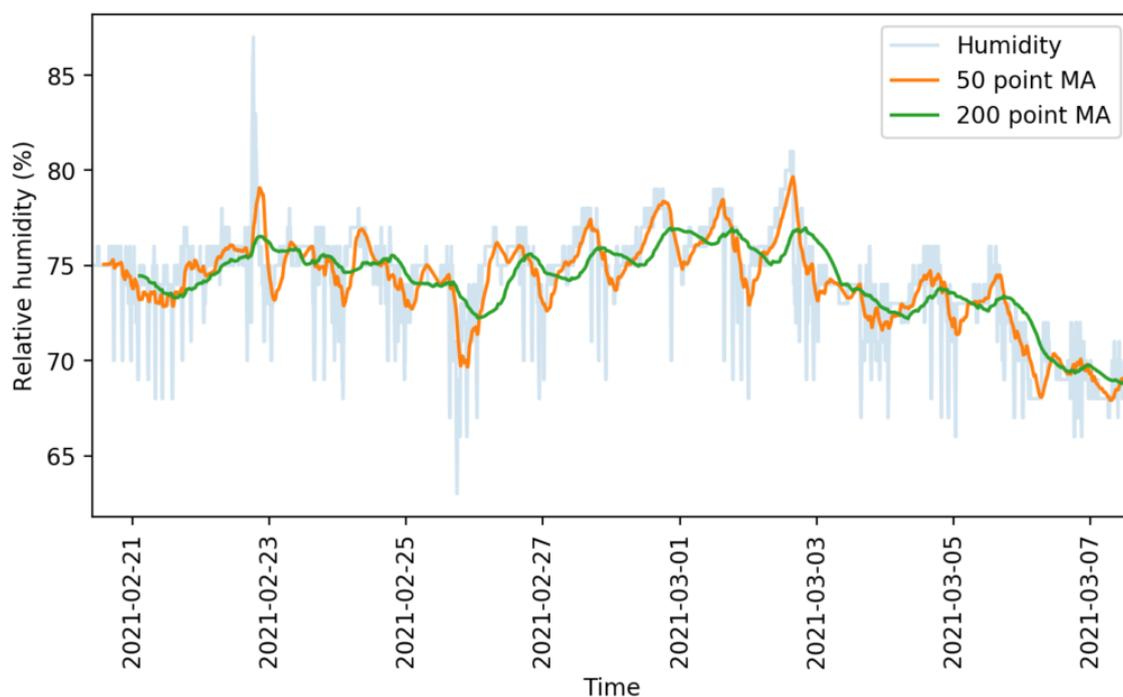
Use of different moving average to smooth out sensor readings. The lowest hanging fruit to take advantage of logged data is to be able to download the data and put it into a database structure that you can properly query and search. Most data logging solutions record the data in either very simple structures, like csv files, or non-relational databases – like
