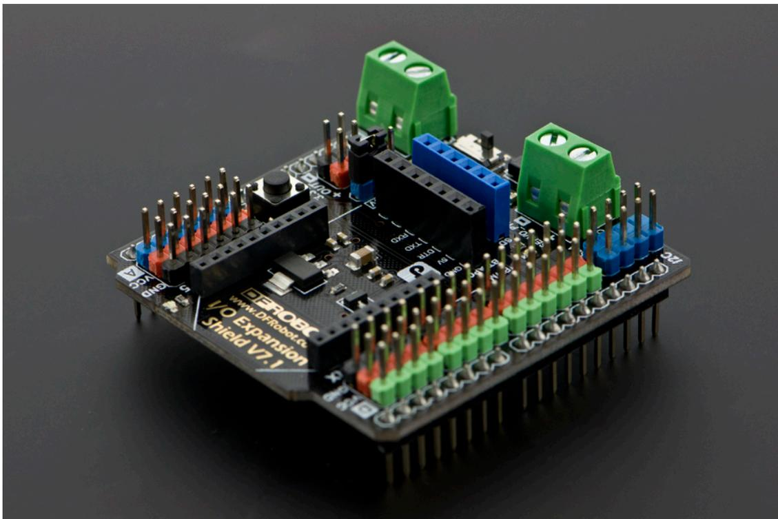
The Gravity I/O shields are an incredibly versatile tool to connect sensors/relays to an Arduino sensing/control station
