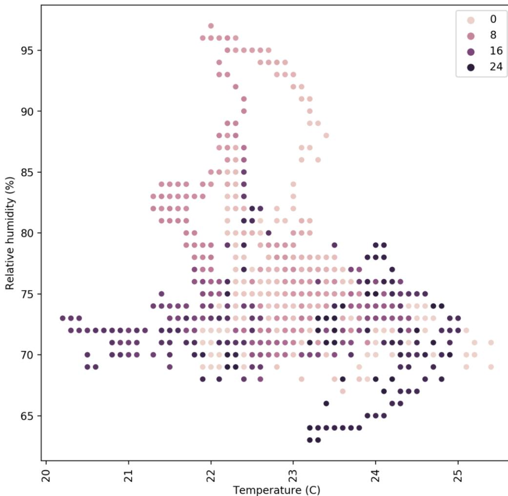
Relative Humidity Vs Temperature map colored as a function of the hour of the day for a growing room being constantly monitored
