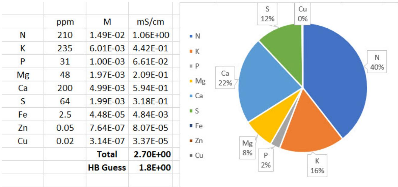
Conductivity calculations carried out by HydroBuddy, also showing conductivity contributions per ion. This is done by converting ppm quantities to moles, then multiplying by limiting molar conductivity values here.
