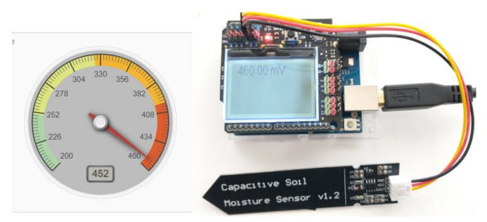
An Arduino Wifi Rev2 connected to a moisture sensor, transmitting readings to an MQTT server hosted by flespi that generates an online dashboard
