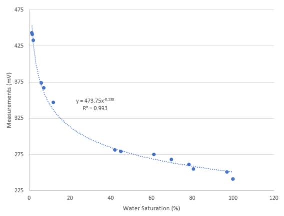
Calibration curve for a capacitive moisture sensor. In this case, the media was a mixture of 50% river sand and 50% rice husks.
