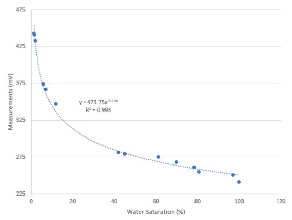
Calibration curve for a capacitive moisture sensor. In this case, the media was a mixture of 50% river sand and 50% rice husks.
