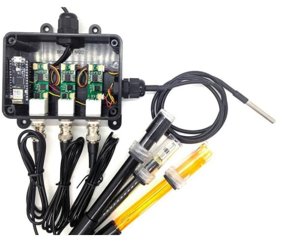
A custom built data logging system to read EC/pH/ORP. Read <u>more here</u>.
