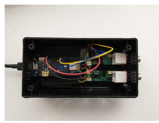
My Arduino MKR wifi 1010 based sensing station, using uFire pH and EC boards in a small project box.
