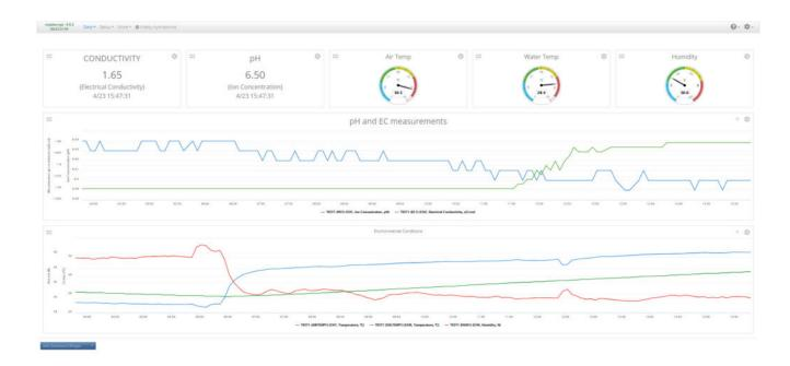
The dashboard of my MyCodo server, showing the measurements of the system as a function of time. All readings are also recorded in the MyCodo database for future reference and processing.
