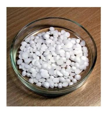
Potassium hydroxide pellets, the most powerful pH up option available to growers
