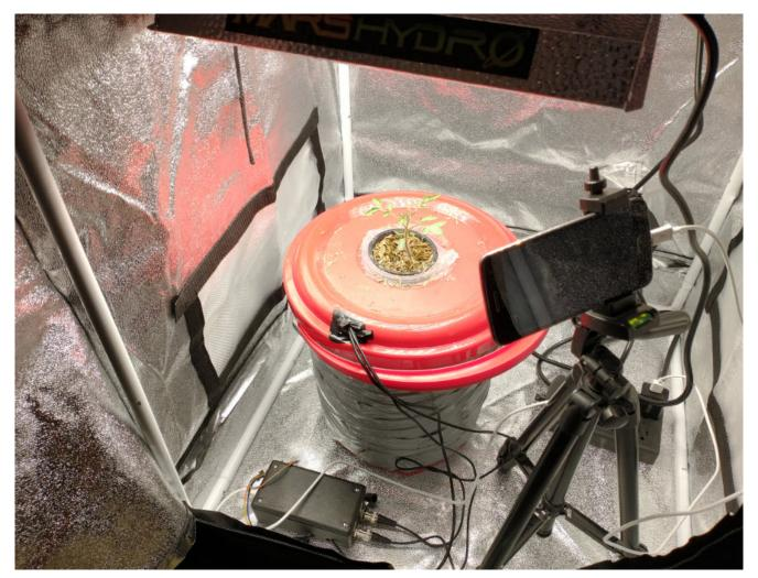
The experimental Kratky setup. You can see the project box housing the Arduino and sensor boards at the bottom. Bernard has been growing for 2 weeks and is already showing its second set of true leaves.
