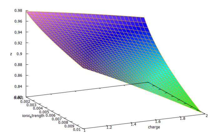
3D plot of equation 4 showing the magnitude of the correction factor (z) as a function of charge and ionic strength.
