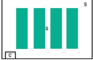
Sensor placement relative to a control source (AC, humidifier/dehumidifier) for one or two sensors. Note that this setup assumes good circulation throughout the room, including middle of canopy.
