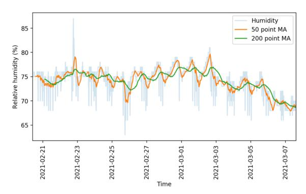
Use of different moving average to smooth out sensor readings.
