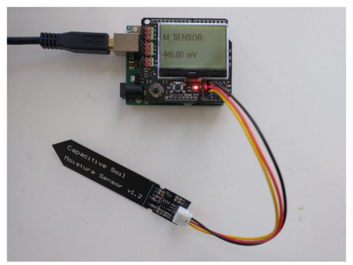
A capacitive sensor plugged into an LCD shield and an Arduino UNO. The measurements are very easy to track with this setup.
