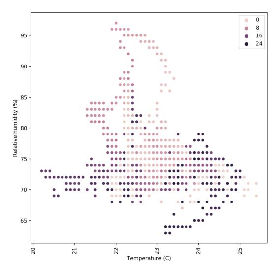
Relative Humidity Vs Temperature map colored as a function of the hour of the day for a growing room being constantly monitored
