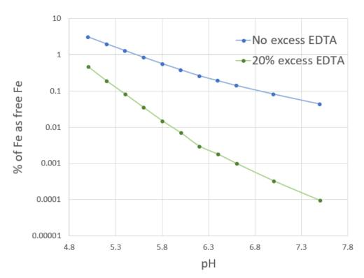
Solution always has 1ppm of Fe added as  $Na_2FeEDTA$  with 30ppm of P. The above was calculated using a system of equations accounting for all the EDTA and phosphate acid/base equilibria, as well as the heavy metal chelation.
