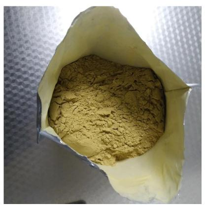
Na<sub>2</sub>FeEDTA, one of the most commonly used Fe chelates in hydroponics.
