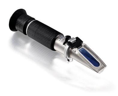
A refractometer, the most common tool to measure brix of plant sap.
