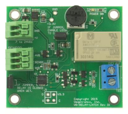
Vegetronix battery powered relay sensor
