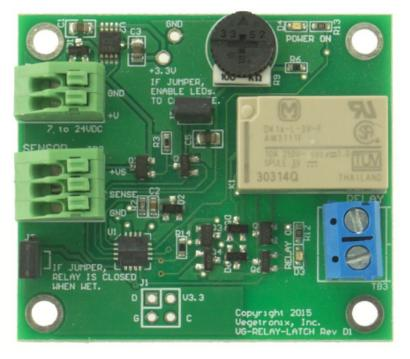
Vegetronix battery powered relay sensor
