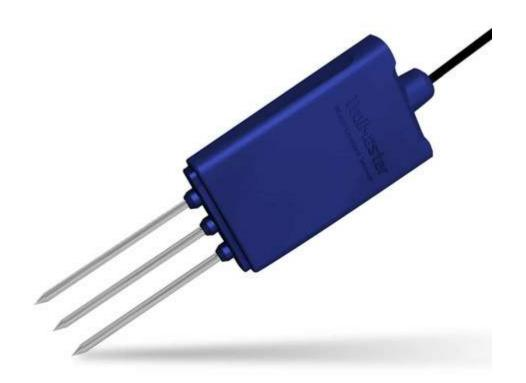
A more advanced resistive sensor that uses AC and stainless steel electrodes to avoid the durability issues faced by cheaper sensors like the one in the previous image.
