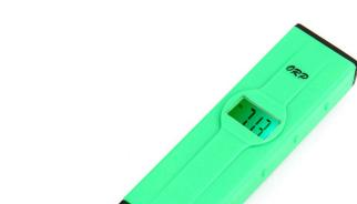
An ORP meter or "Oxidation-Reduction Potential" meter characterizes the electrochemical environment within a solution. An ORP meter has two electrodes, a traditional reference electrode with a known potential and a platinum electrode whose potential changes depending on how hard the solution is pushing either to take electrons from the platinum electron or give it electrons. A solution that has a lot of substances that are willing to give electrons will tend to
