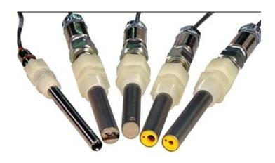
For the grower who wants it all there are also probes like the Mark I-A probe which is a tank-mounted probe assembly that does EC, pH and ORP readings, all in one single fixture. This is incredibly practical since it is able to implement all the readings you need in one single fixture. The problem of course is that calibration of any reading requires you to remove all
