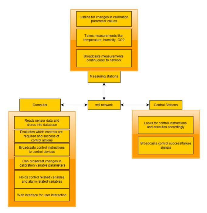
Usual network configuration I used to built electronic monitoring/control infrastructures for hydroponics
