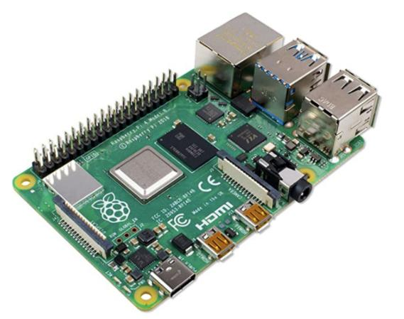
The raspberry Pi 4 computer. Note that you will need a power supply cable and SD card as well, which are an additional cost to the above.
