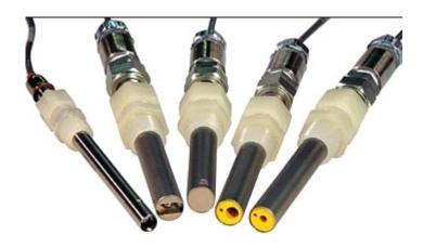
For the grower who wants it all there are also probes like the Mark I-A probe which is a tank-mounted probe assembly that does EC, pH and ORP readings, all in one single fixture. This is incredibly practical since it is able to implement all the readings you need in one single fixture. The problem of course is that calibration of any reading requires you to remove all three sensors so this can be a bit inconvenient when you want
