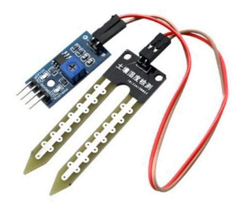
A typical resistivity sensor for measuring moisture content in soil/media
