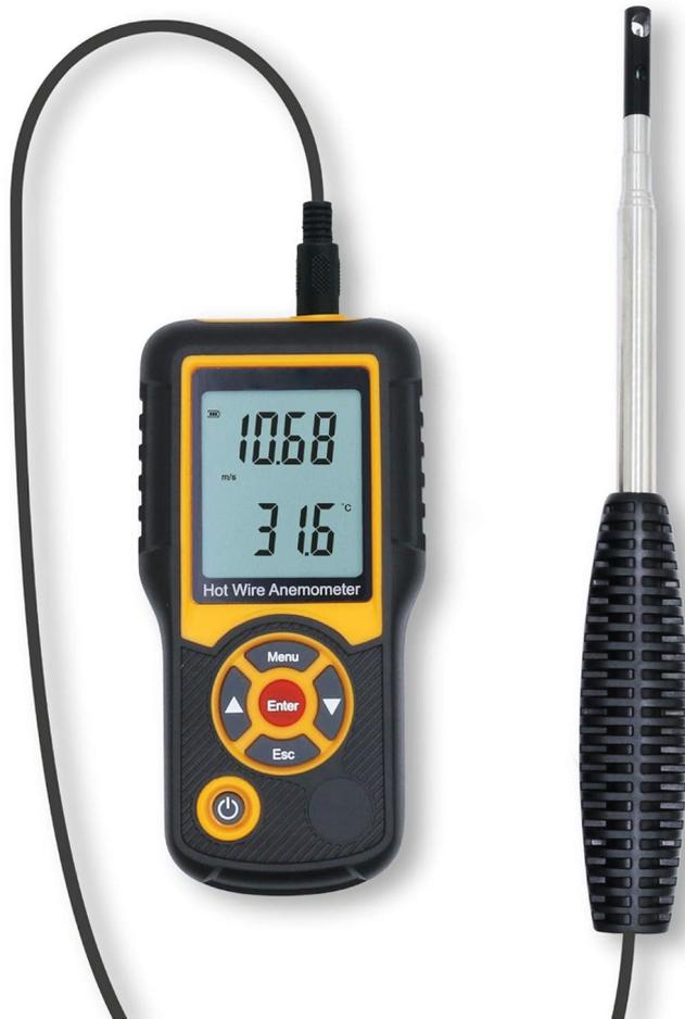
A hot wire anemometer that can be used to accurately measure wind speeds around plant canopy
