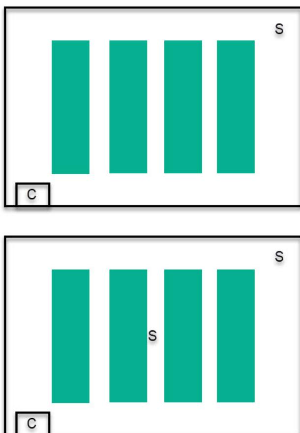
Sensor placement relative to a control source (AC, humidifier/dehumidifier) for one or two sensors. Note that this setup assumes good circulation throughout the room, including middle of canopy.
