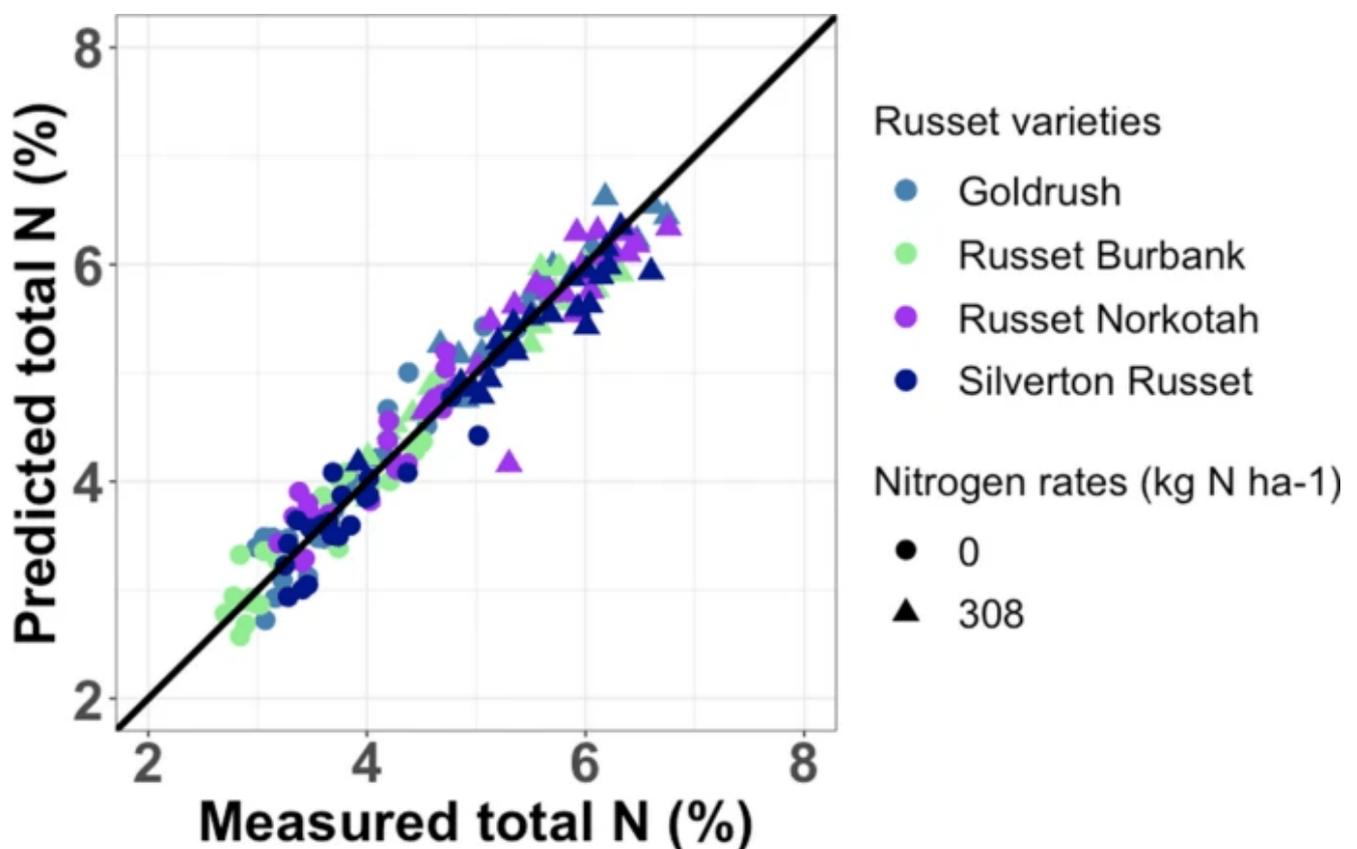
Image showing NIR measured Vs predicted N values for potatoes, taken from ([7](#))
