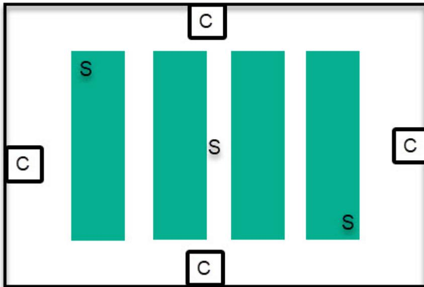
Sensor placement for multiple control sources. Sensors are placed in order trying to always be as far away from sensors as possible but within the plant canopy.
