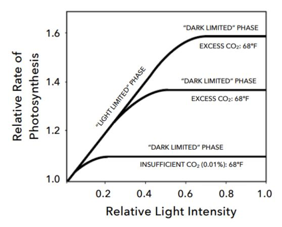
This image illustrates the dependence of photosynthesis on light at different levels of  $\mathrm{CO}_2$  enrichment. was taken from here
